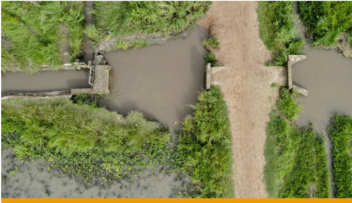
Figure 8: An aerial view of the Tulo Kongwa Irrigation system. The system is unlined, a sign of inefficiency.
