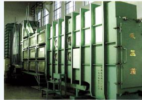
Vacuum tank (vacuum percentage 98.7%; flow discharge 1.0 m<sup>3</sup>/s)
