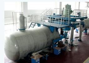
Universal test stand of advanced hydraulic machinery model
