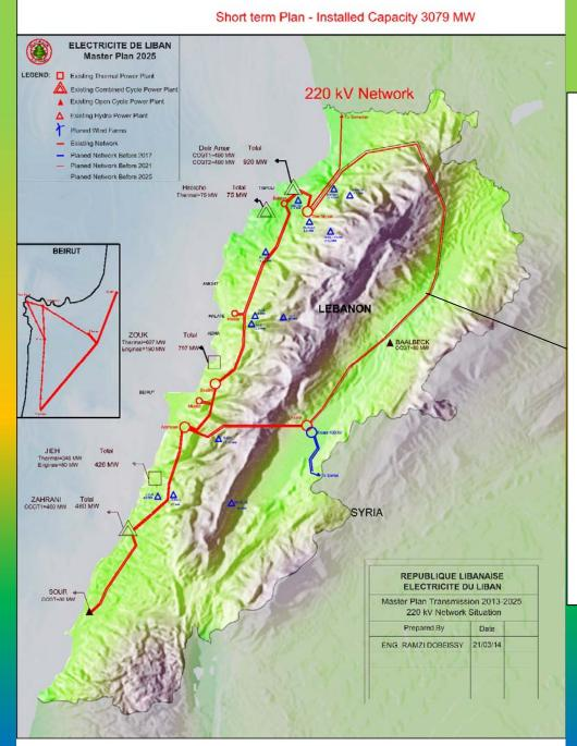
Operate again the second circuit of line Ksara – Deir Nbouh under 220 kV, this will happen soon after the renovation of the 66 kV line which in the last stages. **Ksara-Deir Nbouh** Length = 152 km Voltage= 66 kV Conductor=366mm2 **Almelek** No of circuits=2
