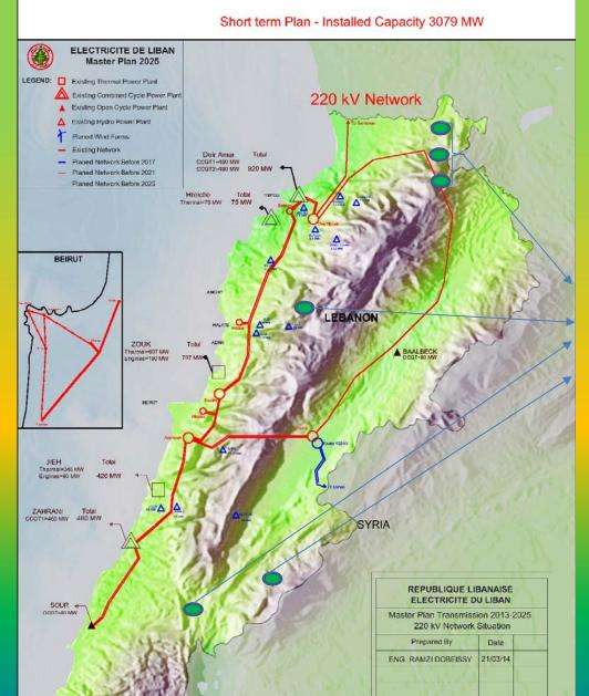
**Expected locations** of "Round Two" Wind Farms based on the wind atlas with an expected installed capacity between 200 to 300 MW, in addition to the three signed Wind **Farms contracts** with an installed capacity of 220 MW in Akkar region.
